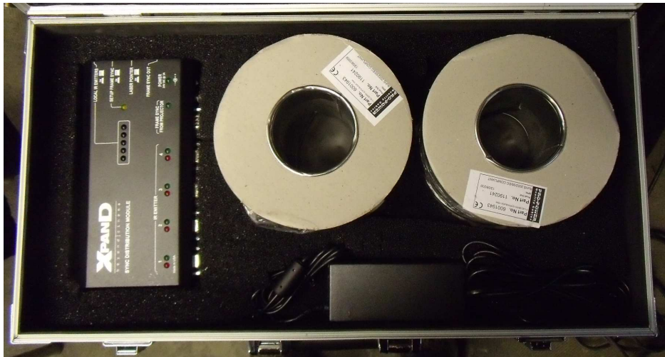
Emitter kit – lower layer – Distribution module, 2 x emitter cables, power supply
