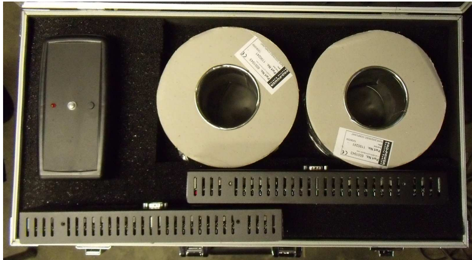
Emitter kit – upper layer – glasses tester, 2 x long range emitters
